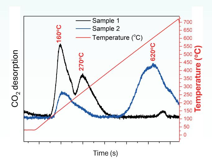
$\rm CO_2$  desorption analysis during heating the solid samples in Argon flow up to 720°C with 10°C/min heating rate. This analysis can be also performed in  $\rm O_2$ -rich gas atmosphere for combustion tests.
