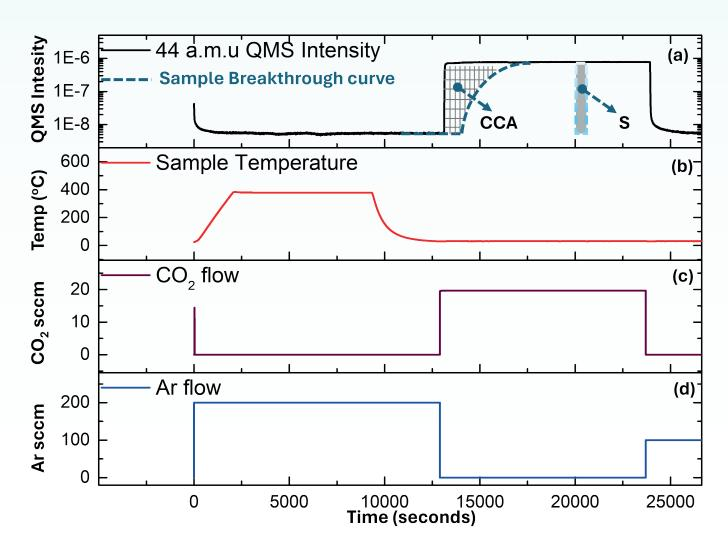
Experimental outputs of each parameter during typical CO<sub>2</sub> capture analysis. (a) CO<sub>2</sub> breakthrough curve based on NDIR CO<sub>2</sub> Sensor, (b) temperature reading from K-type thermocouple standing just 5 mm above the sorbent material, (c) and (d) CO<sub>2</sub> and Ar gas flow in sccm during the analysis. CCS refers to the CO<sub>2</sub> Capture Area
