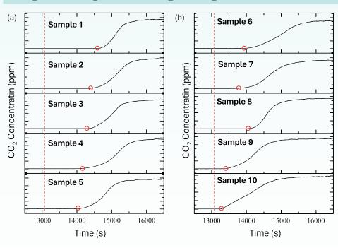
Dynamic CO<sub>2</sub> adsorption breakthrough curves of CO<sub>2</sub> signal recorded by NDIR CO<sub>2</sub> Sensor under continuous 20 sccm 0.2% CO<sub>2</sub> gas flow of ten different test samples. Red dashed-line vertical to the x axis corresponds to gas switch onset point from Ar to 0.2% CO<sub>2</sub>. Red circles pinned on CO2 curve represents the point where CO2 signal rise up.
